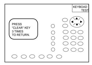
Figure 13-5 Keyboard test
